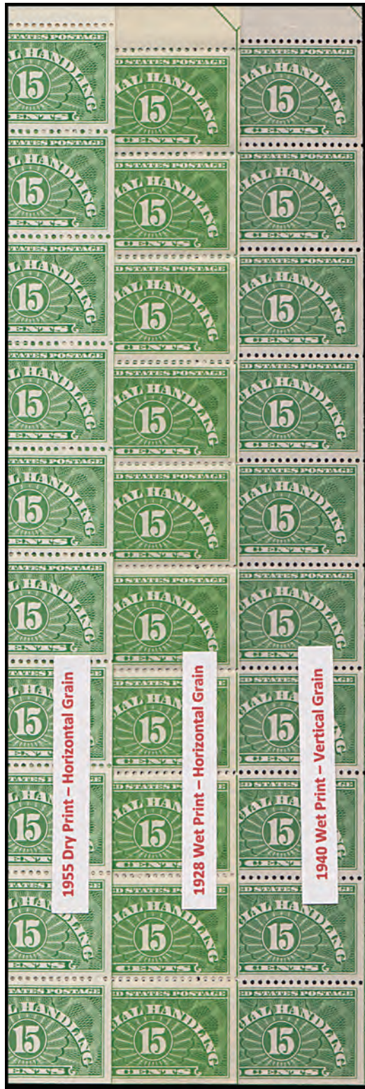
Figure 4. Examples of sheets printed from plate no. 19557 by three different methods illustrating vertical design shrinkage.
