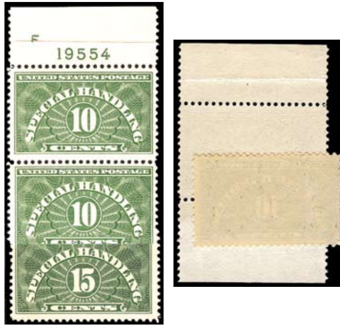
Figure 3. Left: dry-print 10¢ pair with plate number 19554, trimmed horizontally at bottom for use as a template, superimposed on wet-printed 15¢ stamp. Right: same dry-print pair, gum side, soaked off lower \frac{3}{4} of lower stamp of pair to show the white paper and to measure caliper; wet-print stamp superimposed, showing light-yellow gum.
