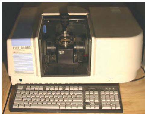
Figure 1. Shimadzu model 8400S spectrometer, fitted with a Pike Miracle sampling accessory. The analyzed portion of the stamp is immediately below the micrometer anvil of the ATR accessory..
